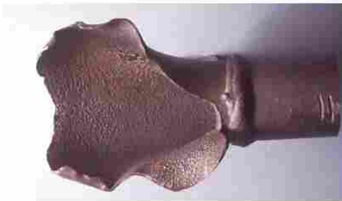
Figure 3-9 FAC Failure and Damage on an Economizer Inlet Header Tube. All HP and LP Heater Tubing in This Unit Was Stainless Steel. The Feedwater Was AVT(R).
